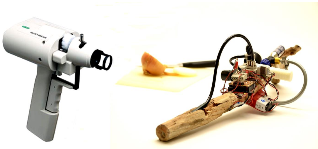
Figure 1. A gene gun, or a biolistic particle delivery system, originally designed for plant transformation, is a device for injecting cells with genetic information. This technique was developed as an alternative to other, more traditional, genetic material transfection methods. The technique fires microparticles that insert the desoxy (or rybo)-nucleic-acid into the target cells. The Helios® Bio-Rad gene gun, shown on the left, is one of the most popular choices in biotechnology laboratories using bioballistics. The one on the right is also a gene gun hacked by Rüdiger Trojok, a biohacker. As the Bio-Rad solution is integrated into scientific research technological problem solving (e.g. O'Brien, Holt et al. , 2001; O'Brien, Lummis, 2011), Rüdiger's hacking is presented as an effective way to have access to this technology, so as to perform a basic transfection into onion cells. The hacked gene gun, shared without peer-review with other biohackers can be built spending 50 EUR, while the professional one from Bio-rad can be sold for up to 15,000 EUR (Trojok, 2012).
